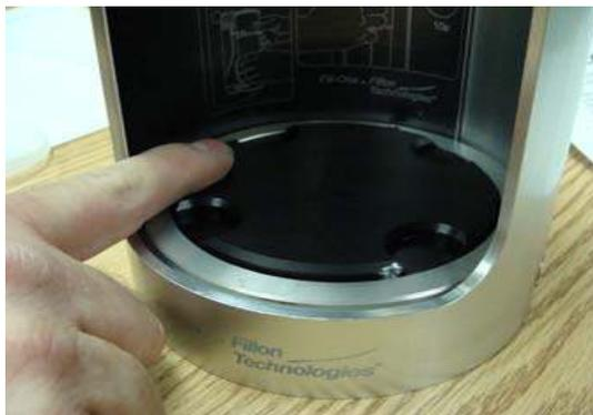
Close the door, then begin cranking the handle until it reaches its lowest position, then crank the handle in the reverse direction until it reaches its highest position. Open the door, loosen the black base plate, and remove the can/cup from the machine. Separate the metal reservoir cup from the can.
