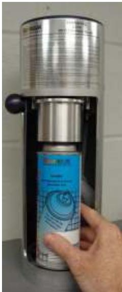
Gently place the reservoir and can into the filling machine, keeping them connected at all times. Slide the brim of the reservoir cup into the reservoir slot. Rotate the black base counterclockwise to snug the connection between the can and cup. Close door.
