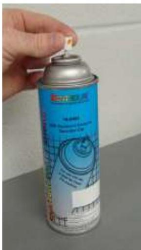
Insert sprayhead using a slight twisting motion with the spray nozzle pointing away from you. Shake can vigorously for 30 seconds to mix the contents. Invert the can and spray for 3 seconds to clear the valve and sprayhead. Place cap back on the can. To fill more cans with the same paint, repeat all steps.
