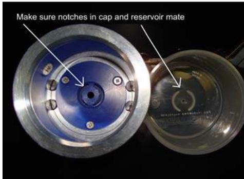
Remove the clear plastic cap from the top of the fill can. Press the metal reservoir cup on top of the can with the smallest opening resting on the top of the fill can. Slide the cap into the metal reservoir cup, so that it mates with the bottom of the cup. Using your index finger, press the bottom of the plastic cap into the bottom of the reservoir cup to ensure a snug fit.
