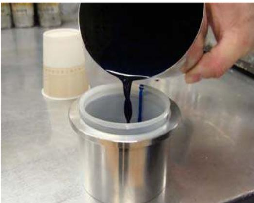
Pour filtered paint to the reservoir cup, **leaving a quarter inch gap at the top unfilled**. Overfilling will cause paint to spill out during the filling process.
